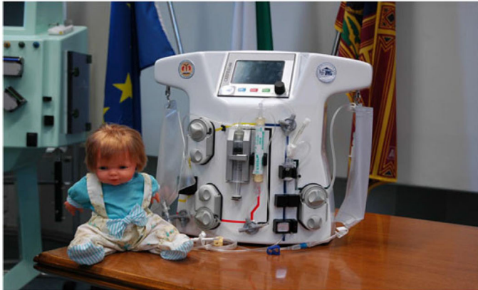
Fig. 3 The C ardio- R enal, P ediatric D ialysis E mergency M achine (CARPEDIEM) measures 44 (L) × 43 (H) × 23 (W) cm, weighs 13 kg, and is specifically designed as a miniaturized, transportable device
